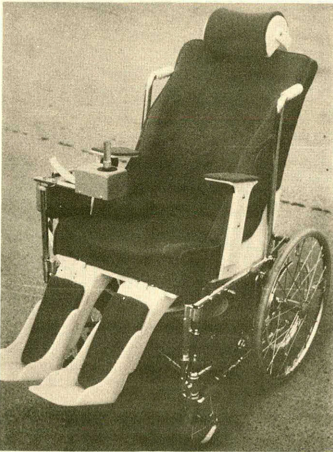
FIGURE 1. Spinal Support System on modified powered wheelchair base. Front view. Armrests and footrests are adjustable and removable.
