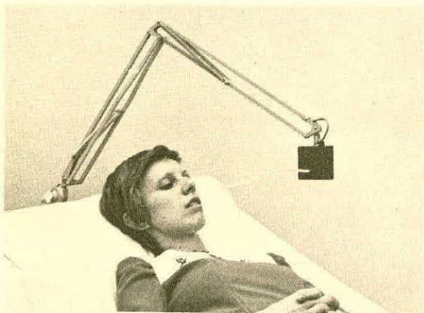
Fig. 1. Picture of simple "call" system mounted on bed.
