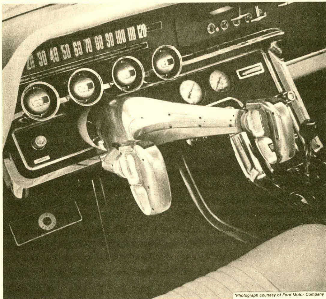
Fig. 3 Example of a pistol grip type integral hand control
