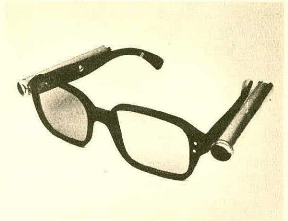
Figure 3. Self-contained non-ranging eyeglass-mounted infrared mobility aid.
