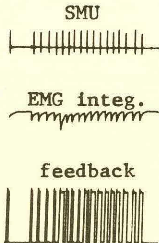
Fig. 2. The Mini-trainer triggering from a single motor unit picked up through surface electrodes. The raw and integrated EMG were both recorded from the device's internal circuitry.
